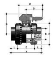
with metric series plain female ends for solvent welding
