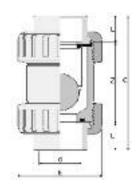
with metric series plain female ends for solvent welding
