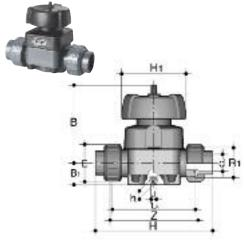
with metric series plain female ends for solvent welding
